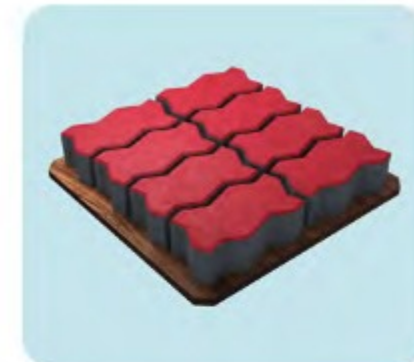
ZIG-ZAG PAVER 225 X 112.5 X 80 (8) Pcs/Hour: 1440 Pcs/Shift: 11,520
